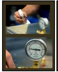
In the final test, the pan gasket is checked for any leakage when the it is torqued to the manufacturer's specifications, heat cycled and then pressurized to 6 psi. (In a real world environment the pan gasket does not see anything more than residual pressure. However, for testing purposes, we pressurized the gaskets to amplify any leak potential.)
