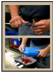
In the first test, Tim measures the percentage of gasket swell for each sample after the material is placed in a transmission fluid bath and heated in an oven at 250° F for 15 hrs. The TransTec® sample shows the least amount of swelling at 7.53%.
